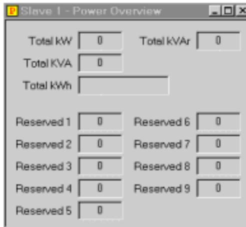
(All fields are double-byte numbers expect for "Total kWh" which is a 32-bit number, it is blank on the screen shot because this feature was disabled on the Access 4000 control panel)
