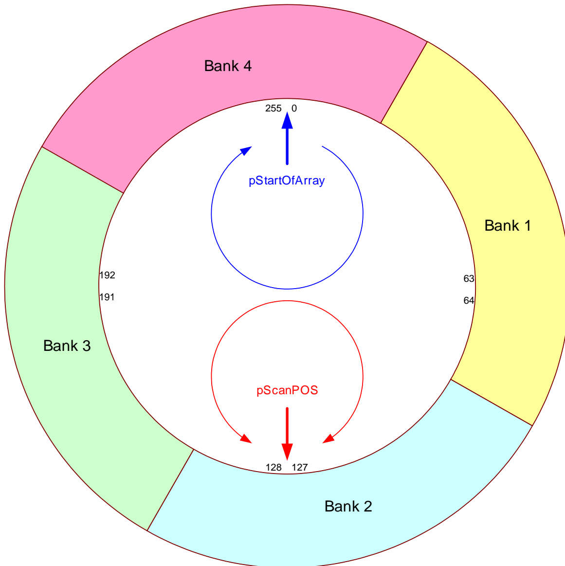
Figure 5.9.2a. Illustration of how time-compressed memory was implemented using internal RAM
